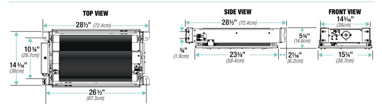
Dimensions - AeroLift 100 with Environmental Air Space Housing & Closure Pane
